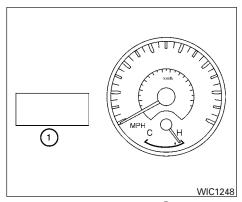
The vehicle information display (1) is located to the left of the speedometer. It displays such items as:
